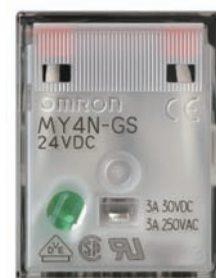
Relay with DC Coil (LED: Green)
